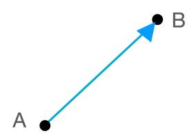
We call A an initial point and B a terminal point with the magnitude represented as  $|\vec{v}|$  and direction represented by an angle  $\theta$ .
