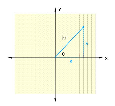
Let a represent the horizontal component and b represent the vertical component.
