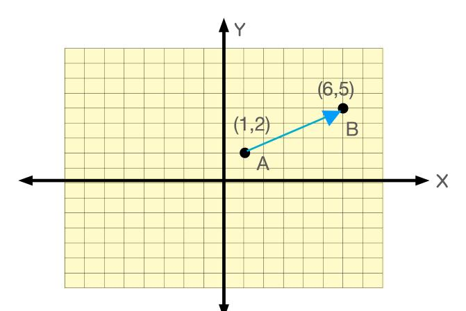
We can determine the **magnitude (length)** of our vector and it's **direction**  $\theta$  by considering two quantities. The horizontal component of a vector and the vertical component of a vector.
