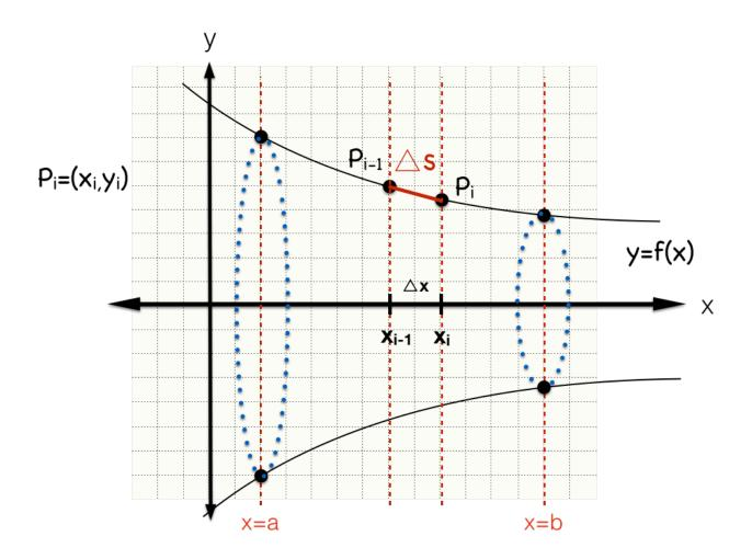
A more detail description of what we obtain by rotating the curve y = f(x) about the x-axis is the ds line segment outlines a conical shape described below in red.
